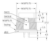
Part No.: MD12P1LPAB Contacts Poles: 12 Pin Connector Gender: Male connector Current Rating: 4 A Keyway Coding: A-Coding EMC Shielding: Half or partial shielded
