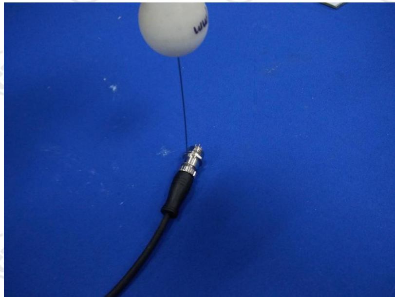
Fig.4- Sample during IP6X test(using test wire of 1.0mm \Phi )
