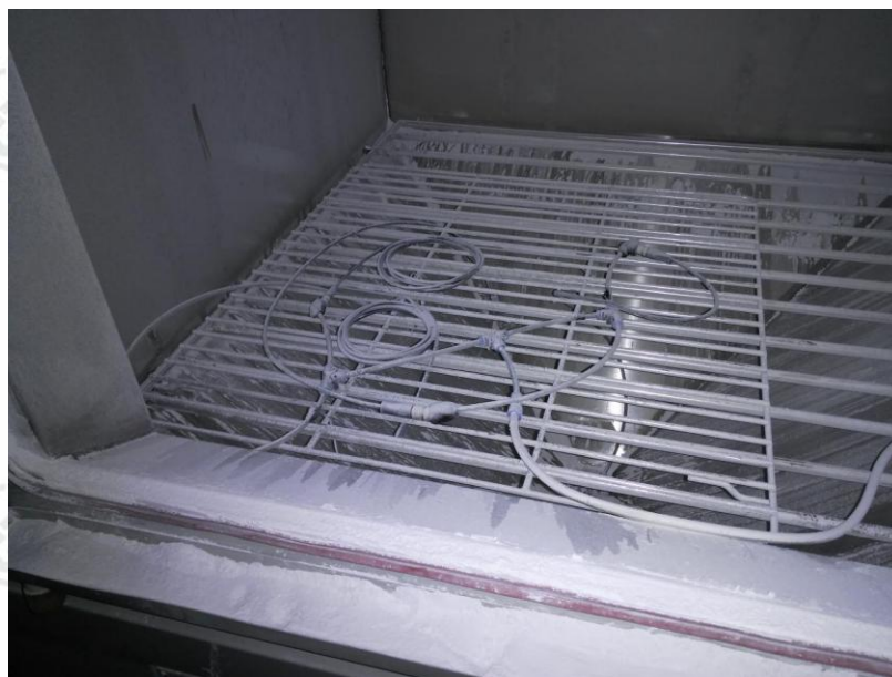
Fig.3- Sample during IP6X test
