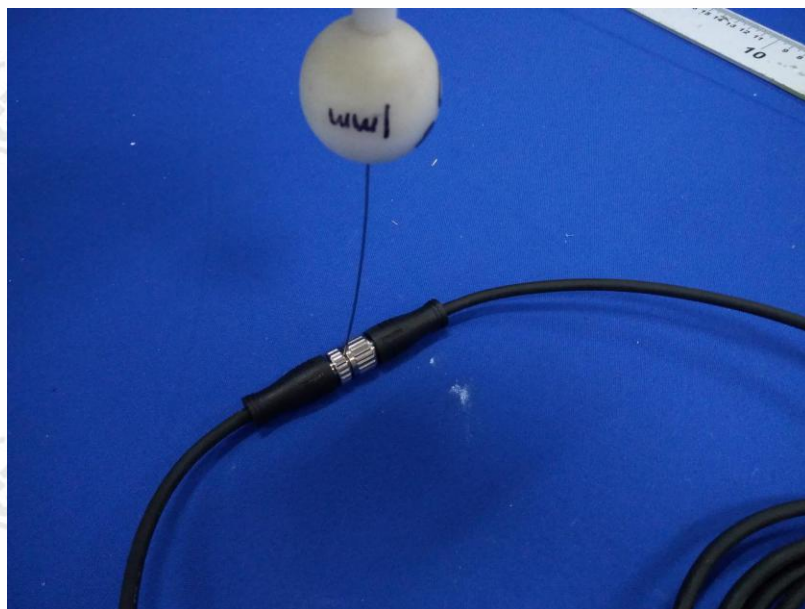
Fig.3- Sample during IP6X test(using test wire of 1.0mm \Phi )
